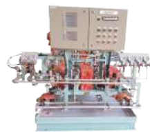
NaOH Dosing Supply System
